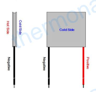
As shown above , when the lead wire is placed in the direction of the user and the red line is to the right, the upper surface of the module is cold side.
